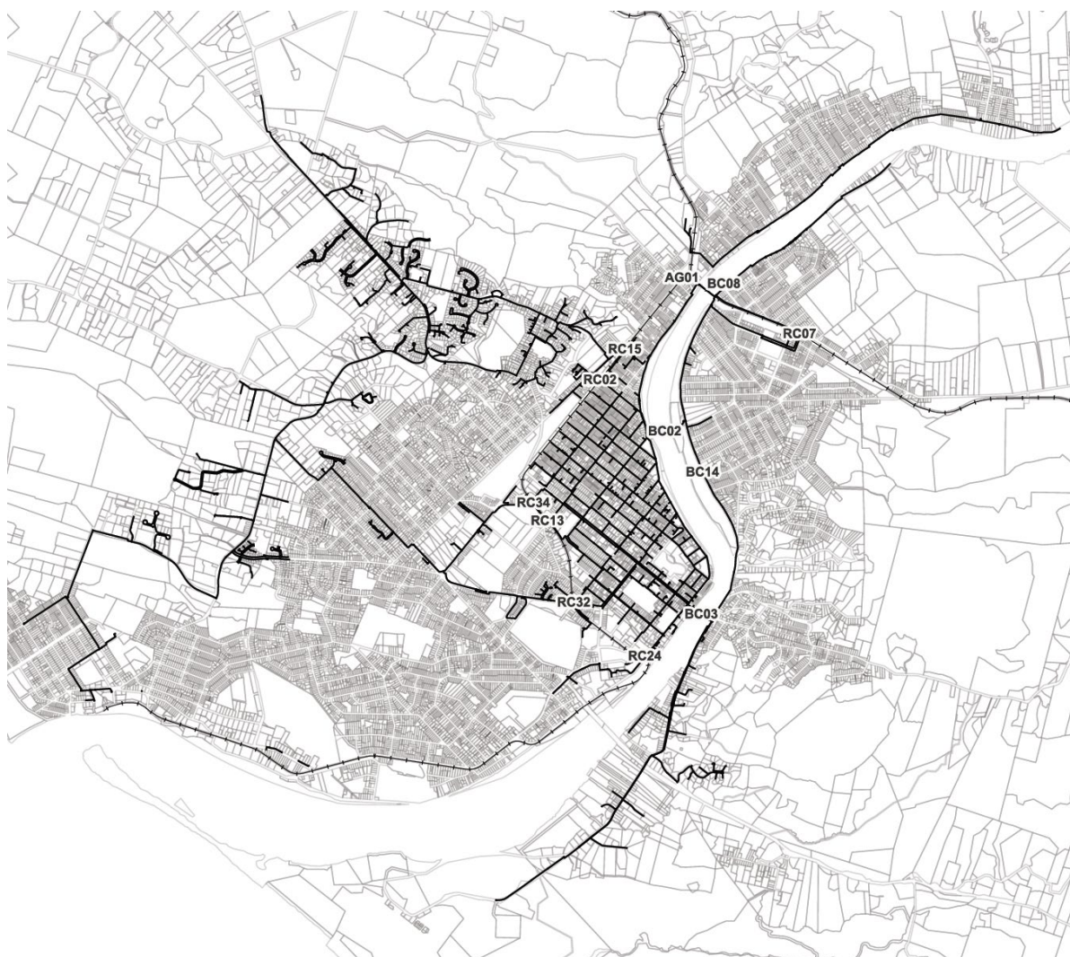
Figure 10: Whanganui Medium Pressure Crossings
