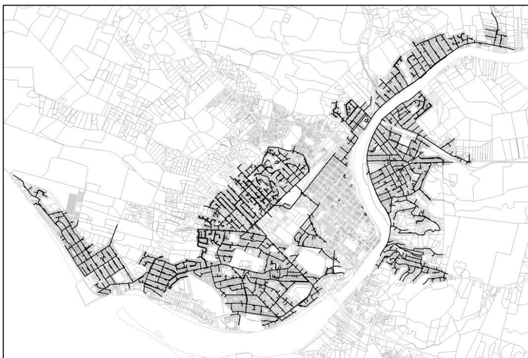
Figure 12: Whanganui Low Pressure System
